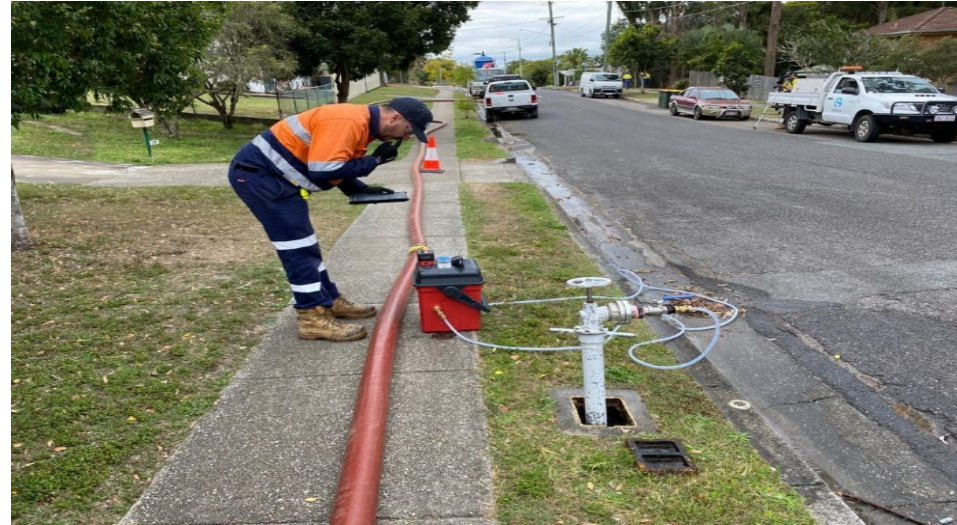
Team Member Recording Turbidity and ORP Measurements
